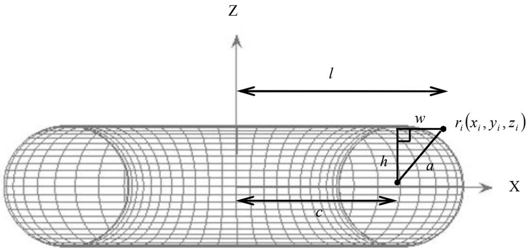
Figure 4. Assessment of torusity error showing minor radius calculation
