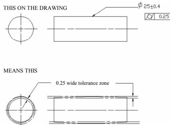
Figure 1. Specifying cylindricity of surface elements (ASME Y14.5M-1994, 1995)
