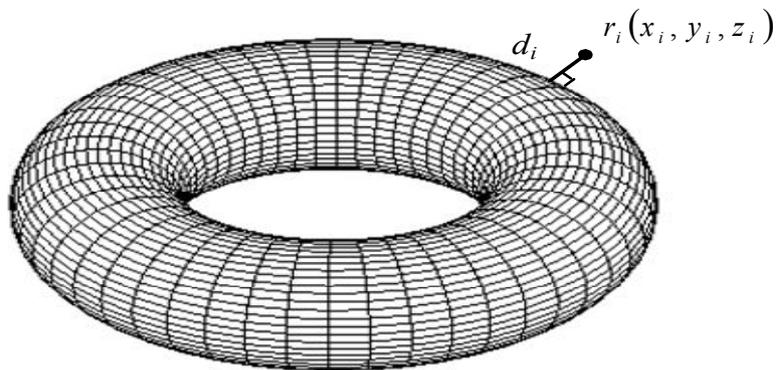
Figure 5. The orthogonal distance from a measurement value  $r_i(x_i, y_i, z_i)$  to the surface of the assessment torus
