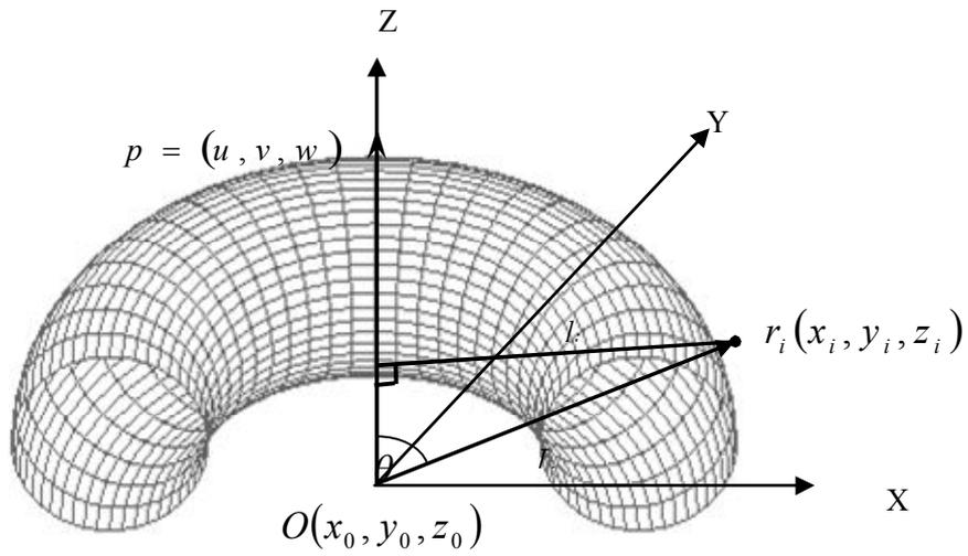
Figure 3. Assessment of torusity error showing calculation of the distance  $l$
