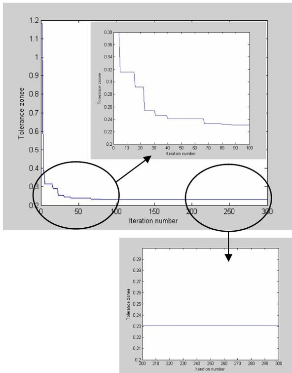
**Figure 7.** Convergence of PSO for Dataset 5 with the closer looks of decreasing torusity from 0-100 and from 200-300 iterations
