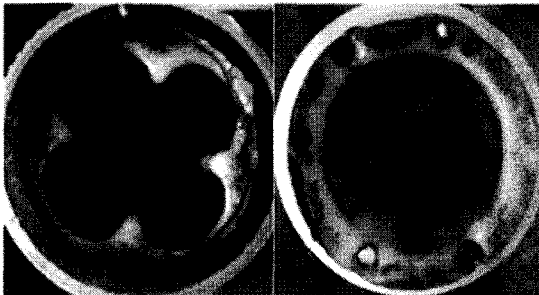
Fig. 2 fuel grains after burning
