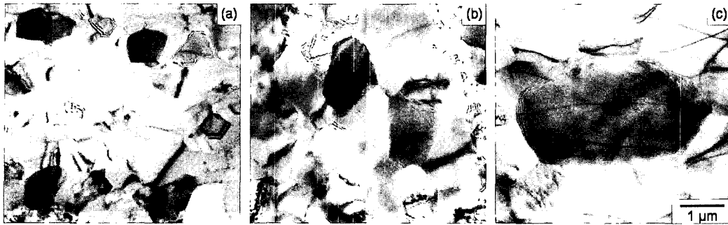
Fig. 3 Transmission electron micrographs of central regions within the friction stir zone of cold-rolled and friction stir processed 1050 aluminum alloy at each tool rotation speed: (a) 560 \text{ min}^{-1} , (b) 980 \text{ min}^{-1} and (c) 1840 \text{ min}^{-1}
