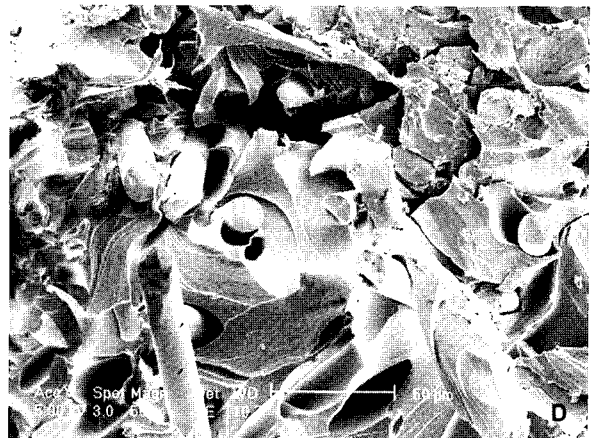
Fig 4. Scanning electron micrographs of the polycarbonate brackets ( \times 500 ). The pattern of the fractured site of Alice bracket wing was quite different from that of Spirit MB bracket wing regardless of thermocycling. A , Alice brackets with no treatment; B , Spirit MB brackets with no treatment; C , Alice brackets with thermocycling; D , Spirit MB brackets with thermocycling.
