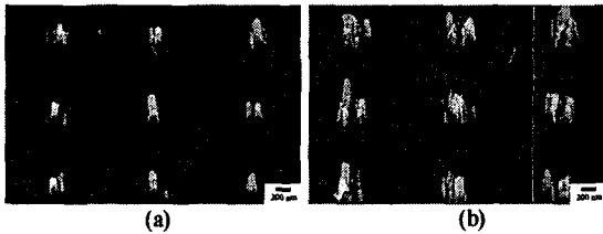
Fig. 11 SEM images of the multi CNTs grown from Ni dots 300 and 400 nm of diameter
