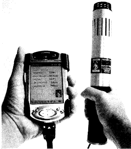
Fig. 5. IAQ monitor for measuring indoor air quality.
