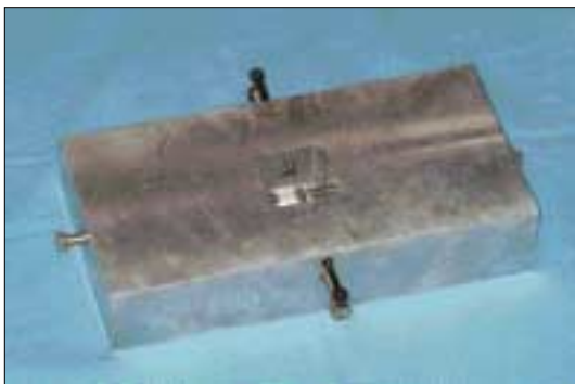
Fig. 1. Aluminum block for stabilizing bone specimen.
