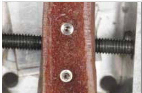
Fig. 2. Bone specimen fixed in aluminum block.
