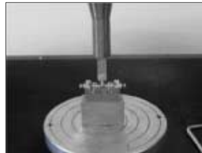
Fig. 5. Jig and specimen used in flexural strength test.
