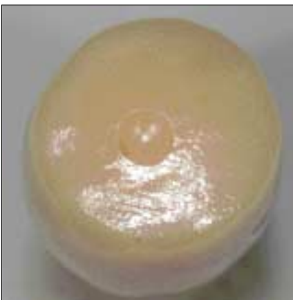
Fig. 2. Spherical indentation on the surface of the metal-ceramic crown sample after cyclic loading.
