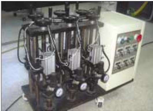
Fig. 7. Universal testing machine. This machine was an impact tester with a pressure gauge attached to the filter controller, and included load cells.
