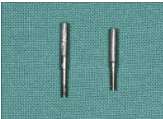
Fig. 1. Experimental ARIPS (anti-rotational inner post system) screws in internal octagons (left) and external hexagons (right).
