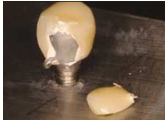
(b) fractured Sinfony-veneered crown.
