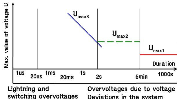
Fig. 5. Maximum value of voltage  $U$  according to duration
