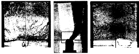
Fig. 11 Fracture path of 3-point CTOD bend test ( \delta=0.719\text{mm} )
