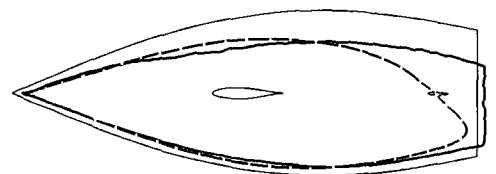
Fig. 17 Waterline shape(Heel: 10 deg., dashed: symmetry, solid: VOF)
