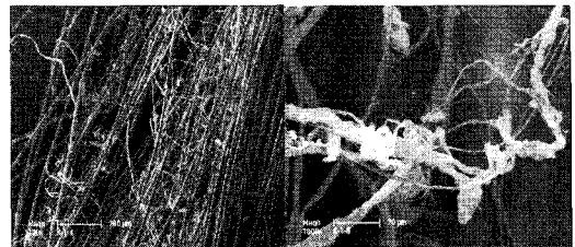
Fig. 7 S.E.M images of torn skin of Kevlar fibers in the form of a helical form.
