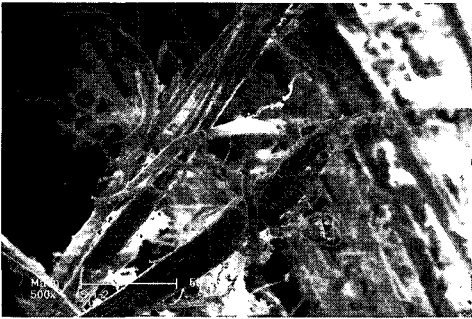
Fig. 12 S.E.M image of fractured Kevlar fibers in STF-Kevlar.
