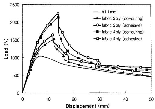
Fig. 9 Experimental load-displacement curves of aluminum-glass fabric/epoxy hybrid tube beams.
