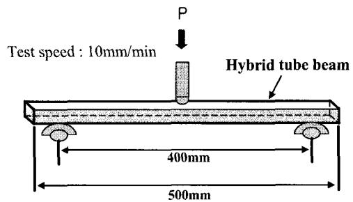
Fig. 5 Schematic diagram of three-point bending test.
