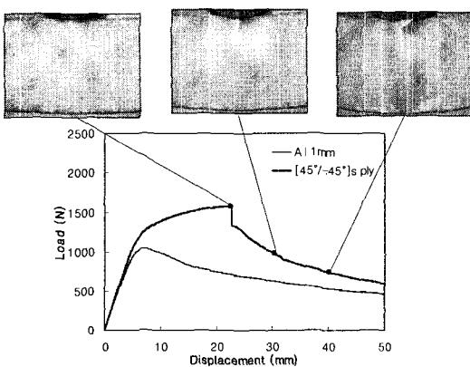
Fig. 13 Experimental load-displacement curve and bending collapse photos of aluminum-UD CFRP [45°/-45°]S hybrid tube beam.
