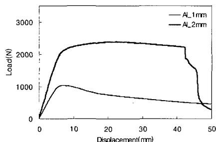
Fig. 2 Experimental load-displacement curves of aluminum tube beams.
