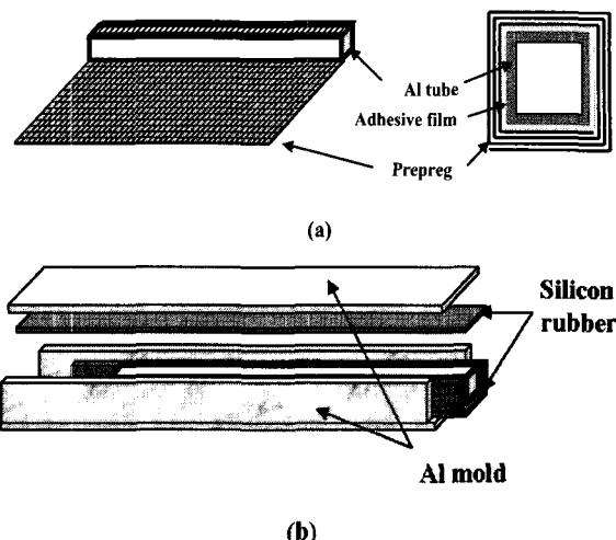
Fig. 3 Manufacturing process for the hybrid tube beams.
