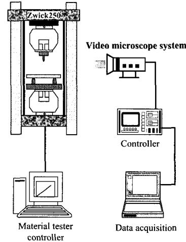
Fig. 6 Experimental set-up for three point bending test.
