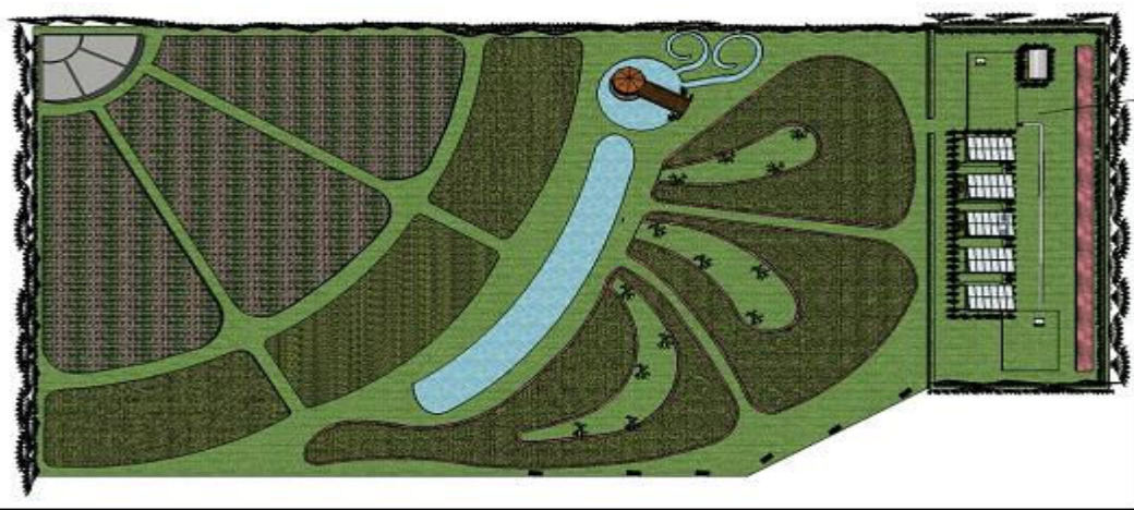
Fig. 5. Schematic diagram of integrated CW system of Phi Phi Island
