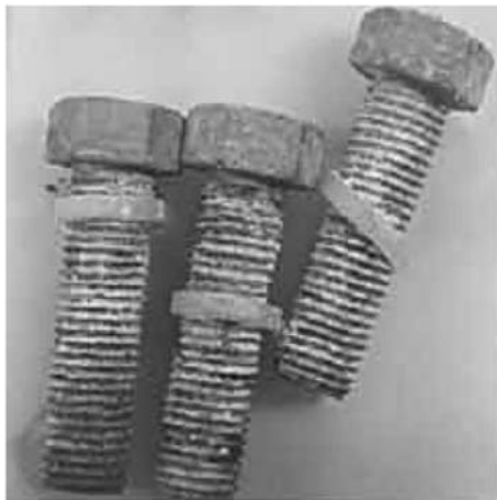
Fig. 4. Feature of initial red rust (with white rust) occurred in M10 bolts after salt spray test (SST; 1500 hour).
