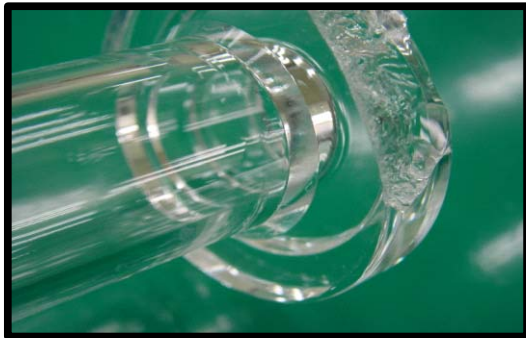
Fig. 15. Macroscopic view of fracture on Fused Quartz Glass happened during process.
