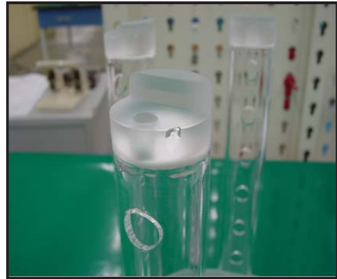
Fig. 2 Pedestal base on which 3 kgf of quartz glass carrier is loaded.
