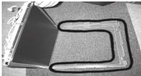
Fig. 2 LCD panel with rubber heater for anti-moisture.
