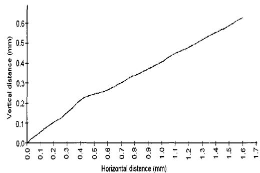
(b) Measured surface profile of the casting part at 15^\circ
