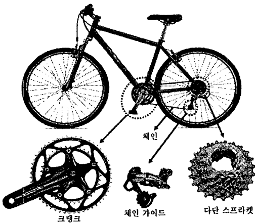
Fig. 1 The components of a bicycle
