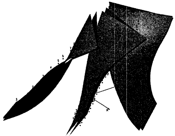
Fig. 18 Comparison CAD model with measuring points
