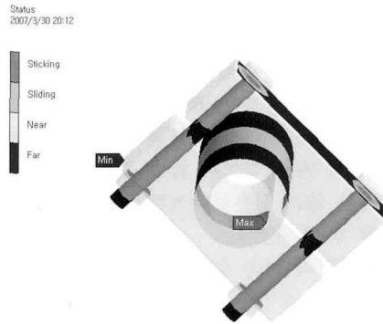
(a) The pipe applied without internal pressure
