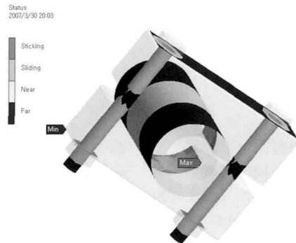
(b) The pipe applied with the internal pressure of 12MPa Fig. 9 Contact state of the contact surfaces
