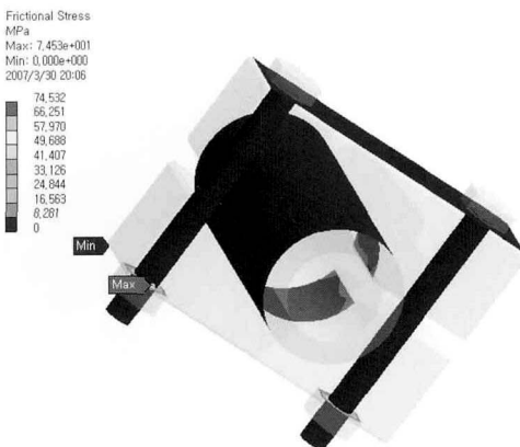
(b) The pipe applied with the internal pressure of 12MPa
