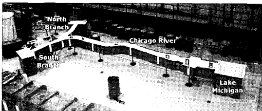
Figure 3. Physical model for Chicago River (Lab's homepage)
