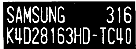
Fig. 3 Binary image using Ostu method
