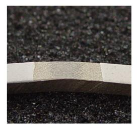
(a) HAp coating on titanium as sprayed
