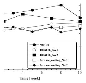
Fig. 4. Changes in corrosion resistance  $(R_c)$  for HAp/titanium combined coatings treated at different cooling rate in physiological saline at room temperature.
