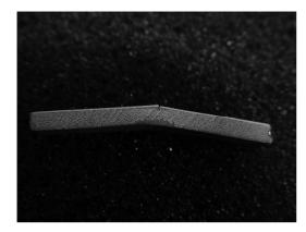
(a) HAp coating on titanium as sprayed
