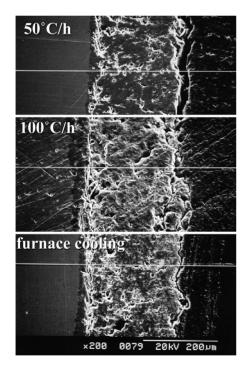
Fig. 5. Cross section profile of plasma spray HAp/titanium coating treated at different cooling rate.
