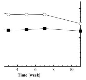
Fig. 1. Changes in corrosion resistance (R<sub>c</sub>) for HAp/titanium combined coatings in physiological saline at room temperature.
