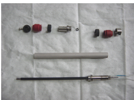
Fig. 3. Schematic design for an anode probe and the actual parts assembled into an anode probe.
