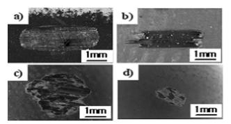
Fig. 9. Wear traces: T800 coating with 610 Hv at; a) 25  $^\circ C$  and b) 538  $^\circ C.$  Sliding ball SUS 304 at; c) 25  $^\circ C$  and d) 538  $^\circ C$
