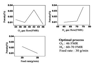
Fig. 6. Porosity of coating vs spray parameters
