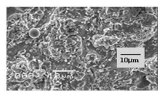
Fig. 2. Microstructure of HVOF T800 coating
