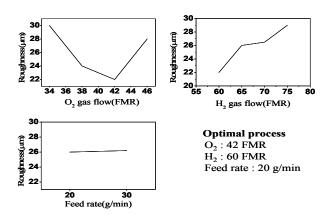
Fig. 5. Roughness of coating vs spray parameters
