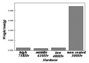
Fig. 8. Weight loss by sliding wear
