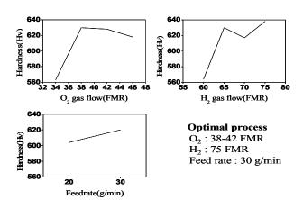
Fig. 4. Hardness of coating vs spray parameters
