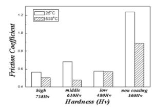
Fig. 7. Friction coefficients of T800 coatings and Inconel 718
