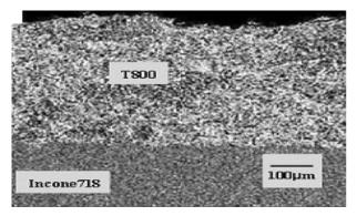
Fig. 3. Cross section of T800 coating on Inconel 718 surface
