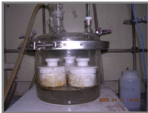
Fig. 3. Soaking test on acid resistance (sulfuric acid)
