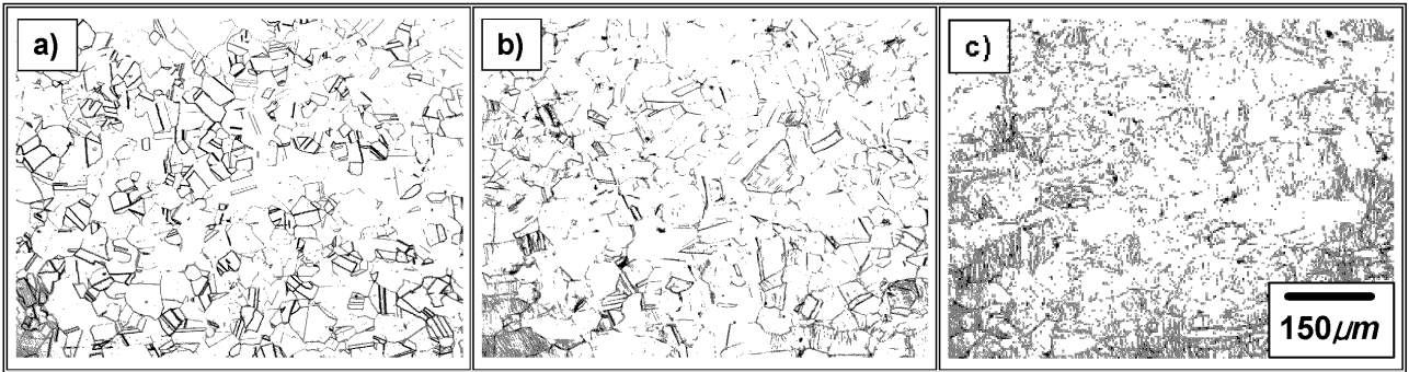
Photo. 1 Optical micrographs of Fe-26Mn-2Al alloy with 70µm grain size (a) As solution treated, (b) After 19.1% cold rolling, (c) After 43% cold rolling
