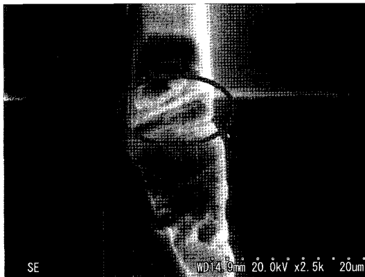
Fig. 7 Micro sized fracture toughness samples showing interlamellar failure with some section of translamellar failure. The image taken at 30° vertical tilt.
