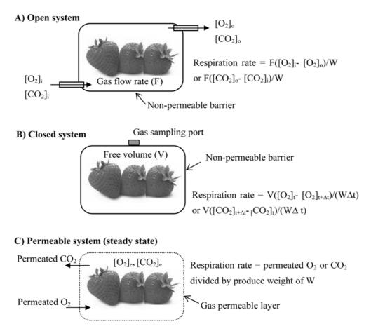
Fig. 1. Schematic diagram for measuring respiration of fresh produce (weight: W).
