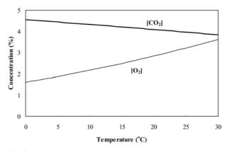
Fig. 4. Equilibrated internal atmosphere of an apple package at different temperatures.
