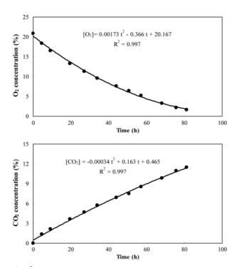
Fig. 2. 2nd order polynomial fitted to the gas concentration data set in Table 1.
