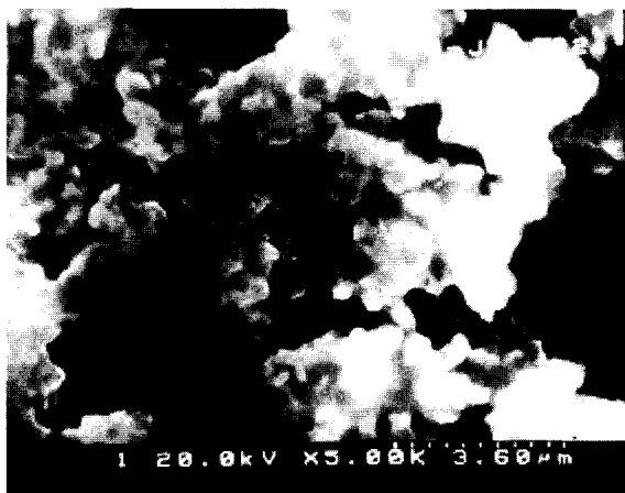
Fig. 4. SEM photograph of the carbonaceous electrode surface of EDLCs.
