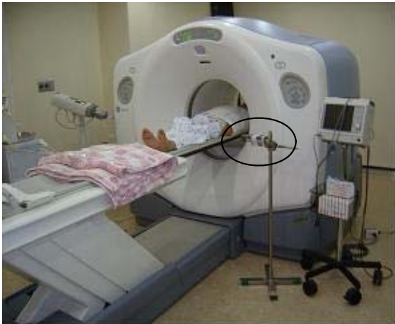
Fig. 2. Experiment equipments of PET and digital surveymeter for apron shielding rates
