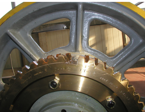
Fig. 5 Broken gear teeth
