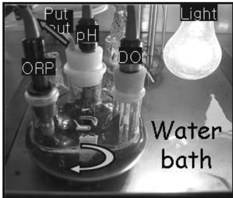
Fig. 1. Apparatus of a 5-neck flask.
