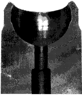
Fig. 7 Cross-sectional view of the developed concave piston assembly
