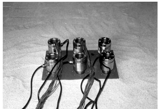
Fig. 4. Load cells connected to pile head
