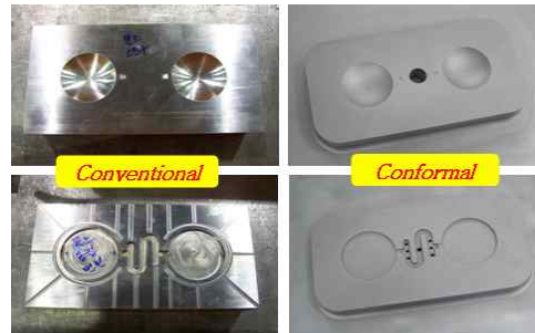
Fig. 5. Photo of conventional mold and rapid mold using DMLS process.
