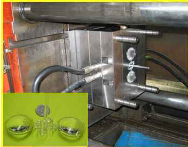
(a) Lens mold installed in the injection molding machine
