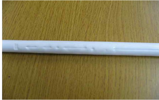
Fig. 2 Detailed sink mark on the central pipe
