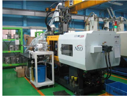
Fig. 6. Injection molding machine for double injection
