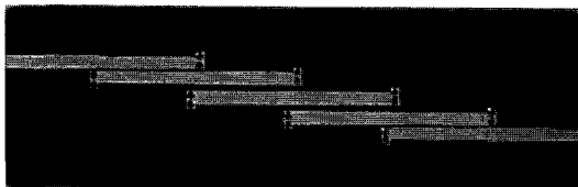
(b) 끝이 접지된 소형화 되지 않은 필터( 45 \times 12 \text{ mm}^2 ) (b) Short ended not miniaturized filter( 45 \times 12 \text{ mm}^2 )
