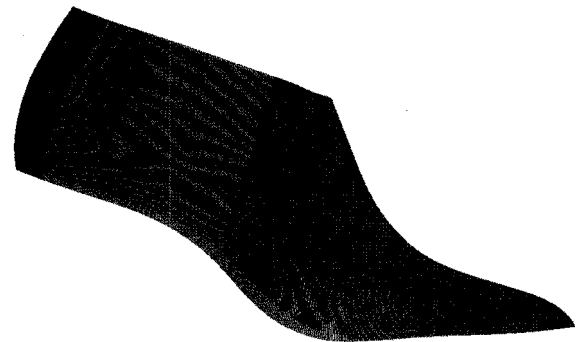
Fig. 9. Point-based model of shoe-last supplied by Clarks International.
