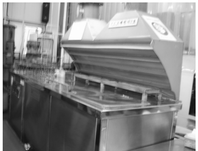
Figure 6. A case on the manual degreasing work by open top degreaser with a lateral hood type of ventilator
