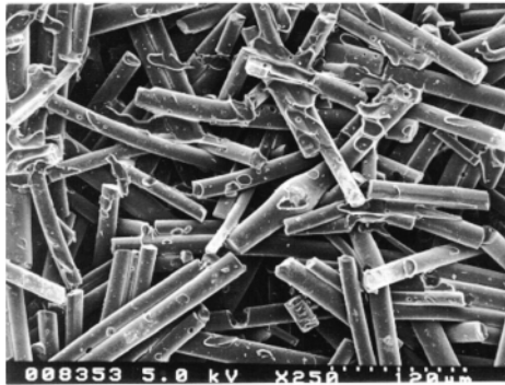
(b) The microstructure of novel gas storage monolith
