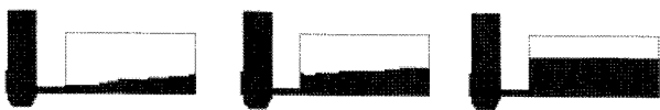
Fig. 4. Flow behaviour during the mold filling (Initial velocity of the molten metal: 23 cm/s, Pressurized system).
