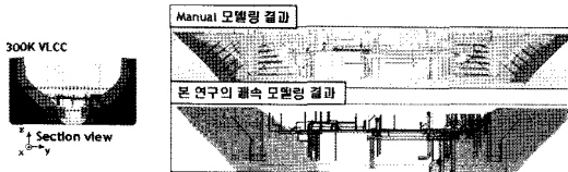
Fig. 11. Result of the pipe modeling of the engine room region of the deadweight 300,000 ton VLCC (section view).
