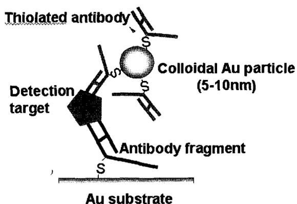
**Fig. 1.** Schematic configuration of immunoassay using the conjugate of Au nanoparticle and antibody fragment.
