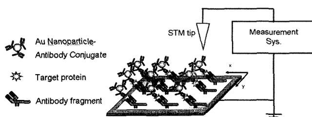
**Fig. 2.** Schematic diagram of scanning tunneling microscopy-based electrical system for detection of protein.
