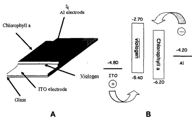
**Fig. 3.** Schematic configuration (A) and energy diagram (B) of the bilayered bio-EL device.
