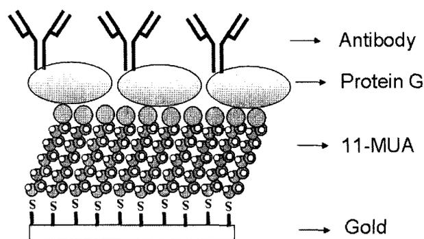
**Fig. 4.** Schematic diagram of the antibody immobilization via protein G on a solid surface by the SA technique.
