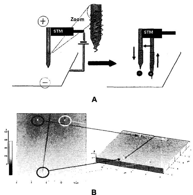
**Fig. 5.** Schematic procedure (A) of DNA nanoarray fabrication using STM and AFM images (B) of a 2×2 DNA array fabricated by STM.
