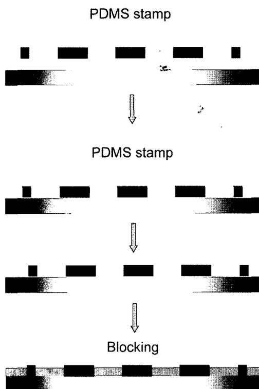
Fig. 6. Schematic procedure of microcontact printing method.
